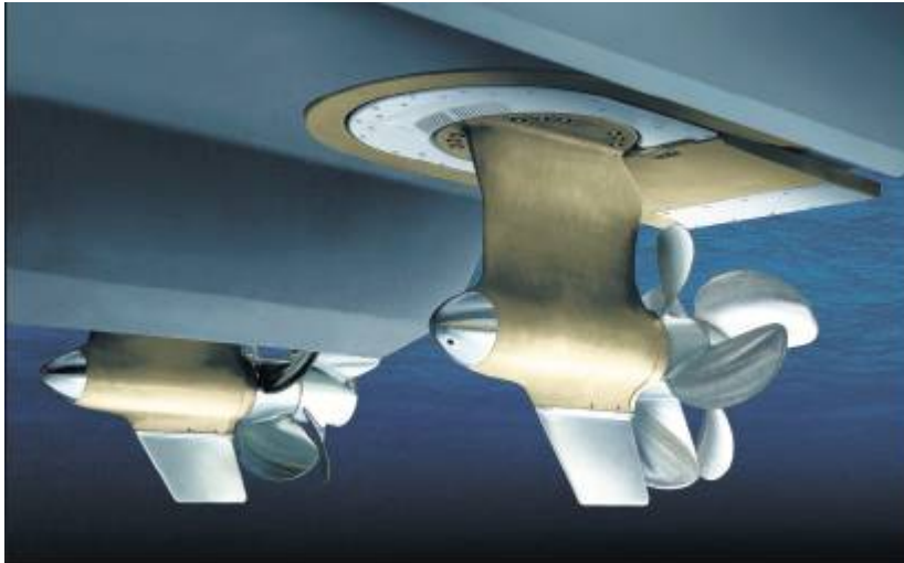
Handling: The Cummins Zeus drive offers excellent manoeuvrability.
